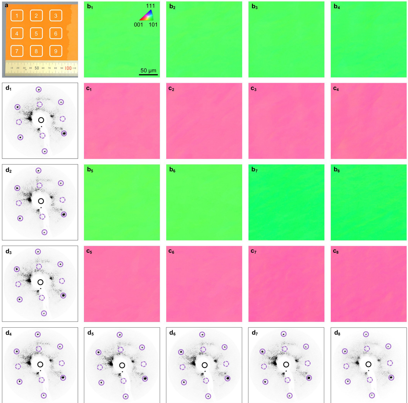
Extended Data Fig. 2 | Characterizations of as-annealed Cu (110) foil at multiple positions. a , Markers 1–9 on the as-annealed Cu foil indicate the positions used for the following characterizations. b , c , Representative EBSD maps along the [001] ( b ) and [010] ( c ) direction measured at positions
